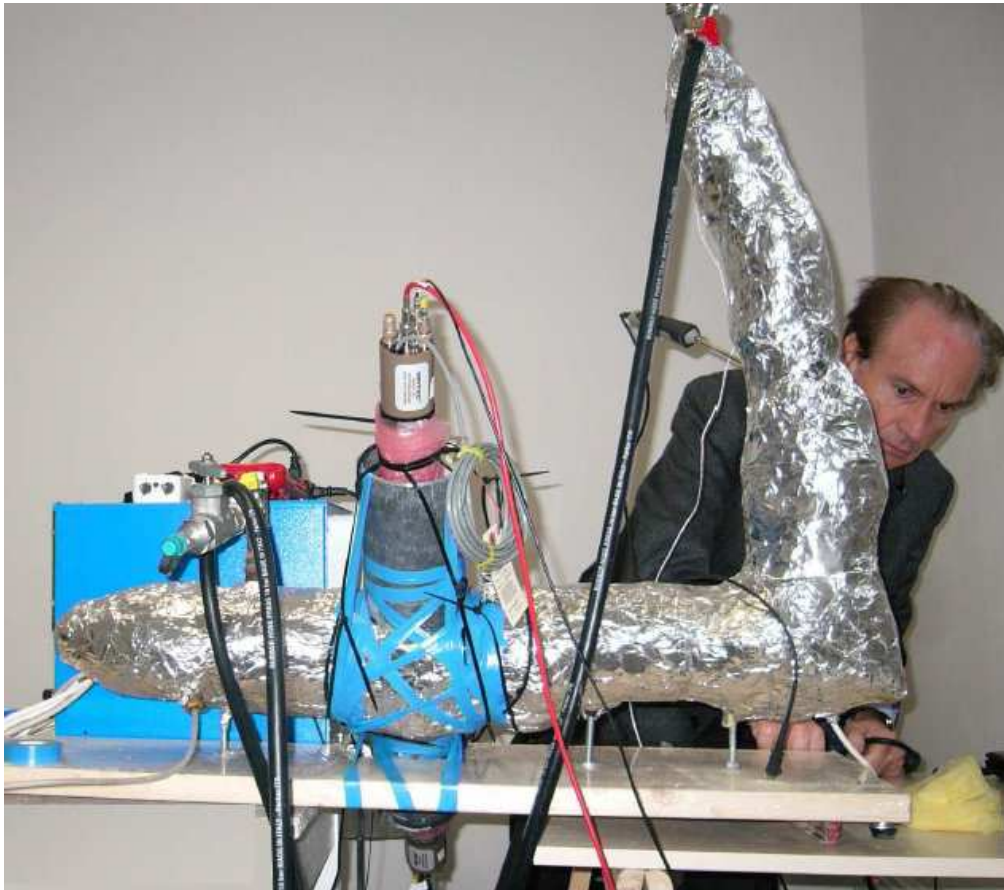
One of the detectors used to reveal the gamma rays at 511 keV. (From the report by M. Villa)
