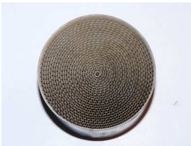
A typical example of a catalyst consisting of a solid substrate, used in cars.
