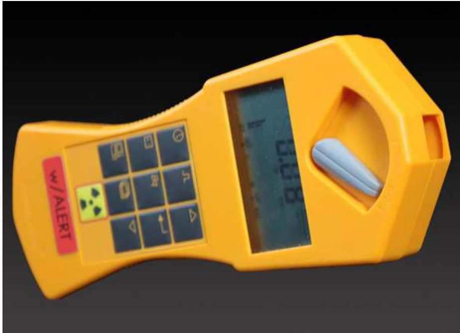
A typical Geiger counter, an instrument that allows you to measure radioactivity.
