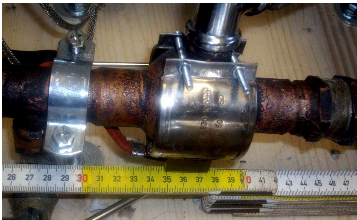
In the foreground, the external resistance enveloping the reaction chamber of an E-Cat.
